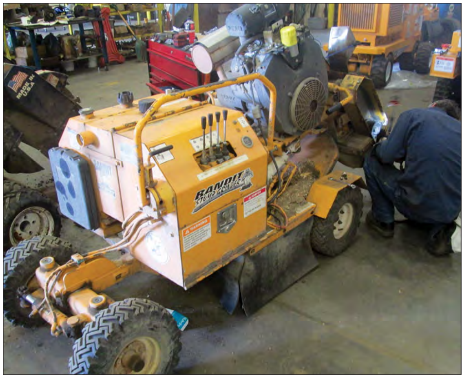
A Bandit stump cutter getting a tune-up. “Longevity depends largely on maintenance,” says Bandit’s Jason Morey. “A tough life will show up over time, all the result of dull cutting teeth, non-adjusted belts or poor engine maintenance.” Courtesy of Bandit.
