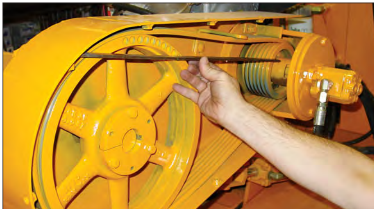
A technician checks the belt tension on a J.P. Carlton stump grinder. “Longevity means keeping belts tight, teeth sharp and bearings greased – all routine maintenance,” says Carlton’s Aaron Foster. Courtesy of J.P. Carlton.
