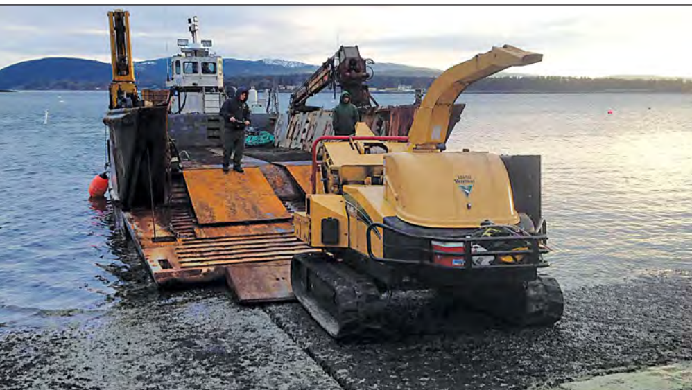
An employee with Savage Forest Enterprise moves a tracked chipper off the barge. Courtesy of Savage Forest Enterprise.
