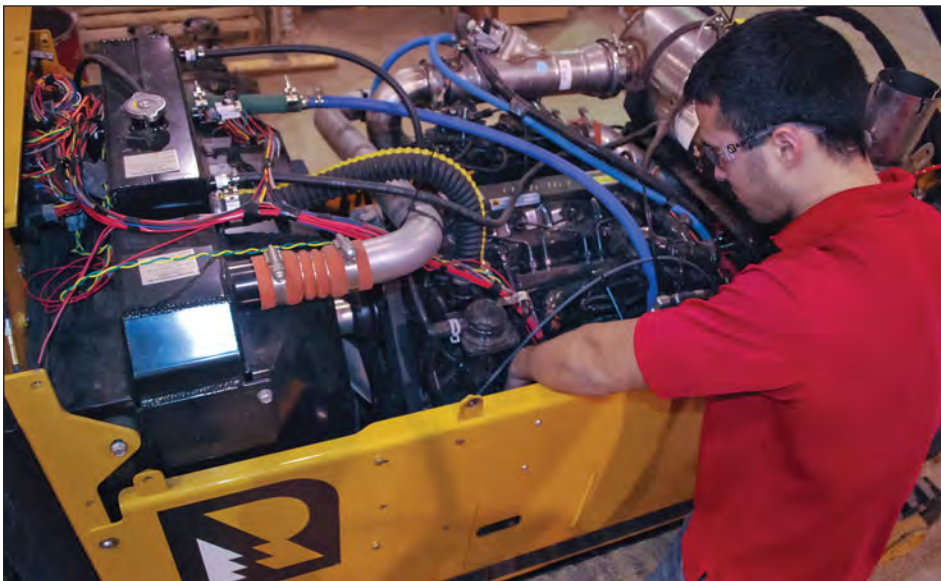
A Rayco technician performs maintenance on a stump grinder. Keeping the machine out of weather when not in use is always a good idea, but even moreso with the mandated Tier IV Final diesel engines – primarily because of the high level of electronics, according to Rayco’s J.R. Bowling. Courtesy of Rayco.
