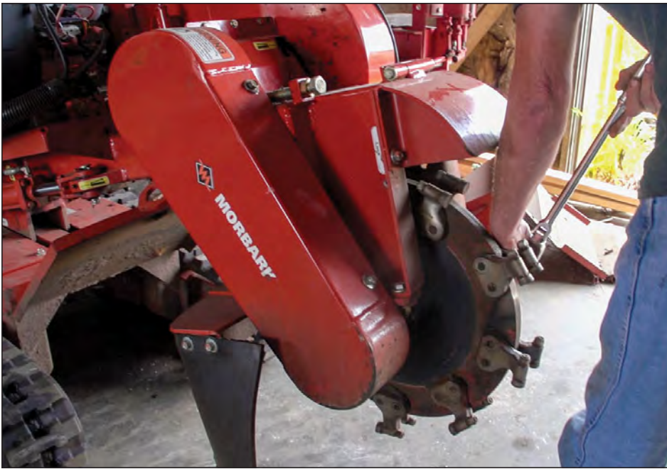
Keeping sharp teeth on the cutter is key to getting the most out of it in every way. “The cutter will work if the teeth are worn, but it pounds the stump, it does not cut it. That puts undue wear on the cutter,” says Morbark’s Casey Gross. Courtesy of Morbark.
